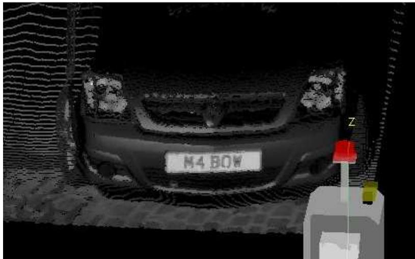
Fig. 21. Close detail of a point cloud built by rendering range and reflectance data from the estimated trajectory of moving Segway platform (New College data set).
